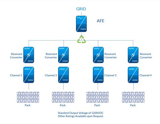
The use of resonant converters for channel to channel isolation provides options for incredibly high efficient battery cycling significantly reducing the test lab operating costs and power requirements. The channel to channel isolation also creates the possibility of putting two of the outputs in series.
